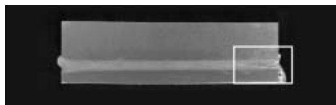
図4 131mm厚アルミニウム合金 EBW溶接部(30kW機) Fig.4 The cross section of aluminum alloy joint welded by 30kW EBW machine (131mm thick)
