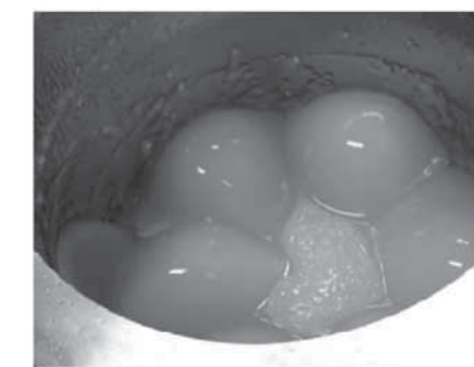
図5 ヒトデ型邪魔板滞留部 Fig.5 Stagnation by baffle for LEVIASTAR
