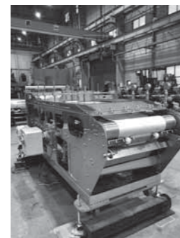
図1-2 販売用テスト装置 Fig.1-2 Horizontal belt filter small-scale test equipment for sale
