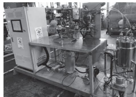
図3 BoCross® フィルタ小型試験機(0.013m 2 ) Fig.3 BoCross® filter small-scale test equipment(0.013m 2 )
