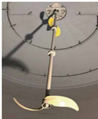
図3 DMBB Fig.3 Appearance of DMBB impeller
