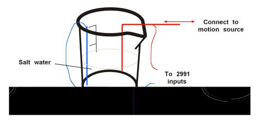
Other linear displacement transducers have been made with two stiff wires suspended in a beaker filled with salt water. One wire (blue above) is fixed; the other (red) is attached to the moving object. Start with just a pinch of table salt, and add until the resistance between the wires at maximum distance is no more than about 2000 ohms.
