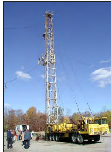
Drill rig and logging truck at CO 2 storage demonstration site in the Michigan Basin.
