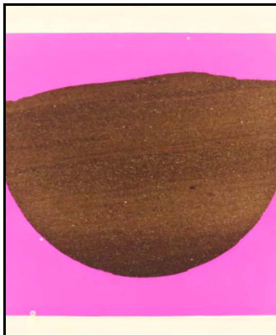
Figure 2. Photograph of Sample G1 thin section. Light and dark bands represent silty (light) versus more clay-rich (dark) laminations.
