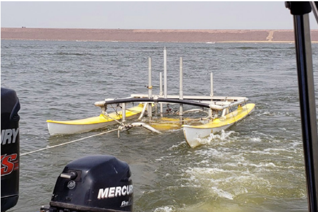
EdgeTech CSS-200 subbottom profiling instrument in tow at Cherry Creek Reservoir in Colorado.
