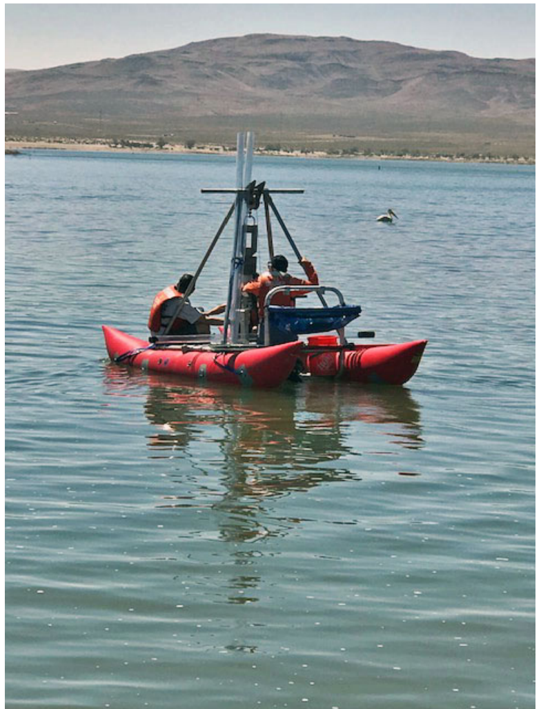
U.S. Geological Survey staff collecting sediment cores from Lahontan Reservoir for dredging water quality impact simulations.
