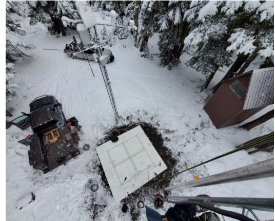
Natural Resources Conservation Service (NRCS) Oregon Snow Survey staff installing an experimental fluidless snow pillow. Photo credit Allen Buckman/NRCS.
