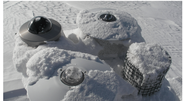
A pyranometer setup near a snowy field (Matsui et al. 2012; used by permission).
