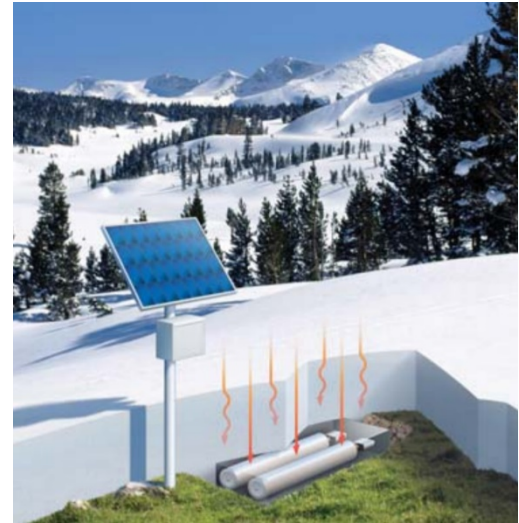
Illustration of Hydroinnova's SnowFox snow water equivalent sensor, installed below the snowpack.
