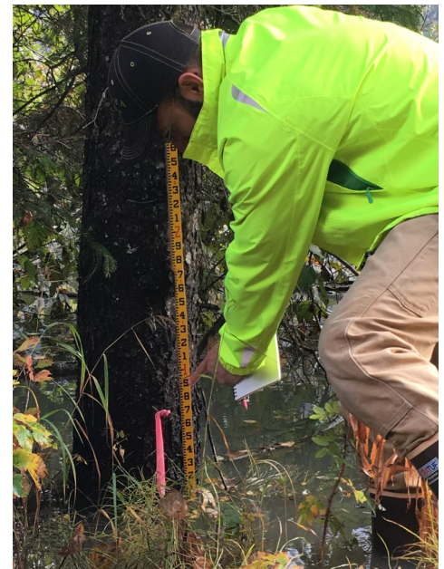
(Left) APRFC Hydrologist Celine van Breukelen (taking picture) explains the ADCP measurement profile to the boat-driver's grandson. (Right) Anchorage NWS Service Hydrologist Andrew Dixon uses pine needles deposited by flood water to determine the high water level near Cooper Landing, Kenai after the Snow GDL outburst. Photo credit: Jessica Cherry, APRFC/NWS.
