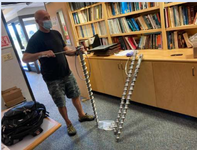
Mike Shanahan with the anchors and wrench used with the new antenna. Photo by Rick Hallman
