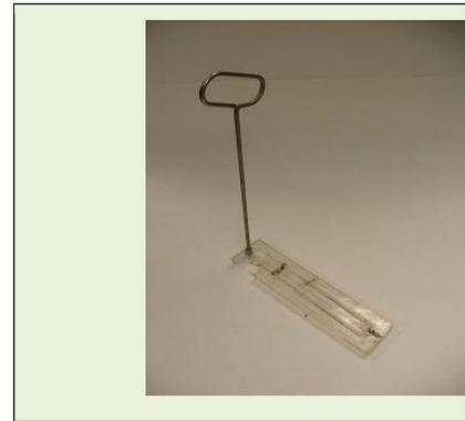
Figure A-29. Submerged Mount Thermometer
