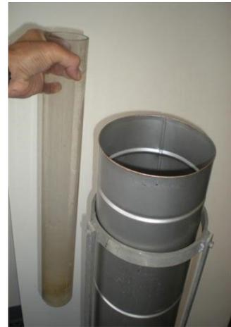
Figure B-10. Removing the Measuring Tube
