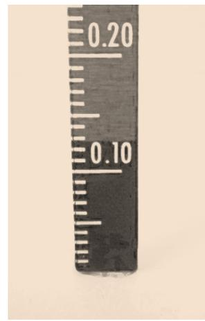
Figure B-13. Reading the Precipitation Amount (0.13)
