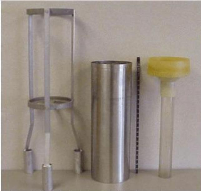
Figure A-4. Eight-Inch Precipitation Gauge Components
