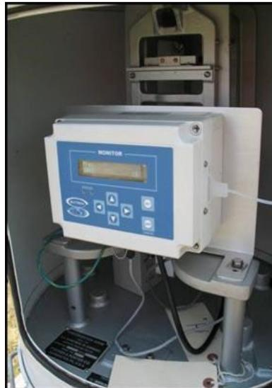
Figure B-20. FPR-D Data Logger
