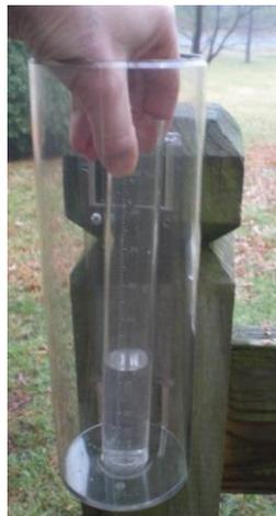
Figure B-6. Removing the Measuring Tube
