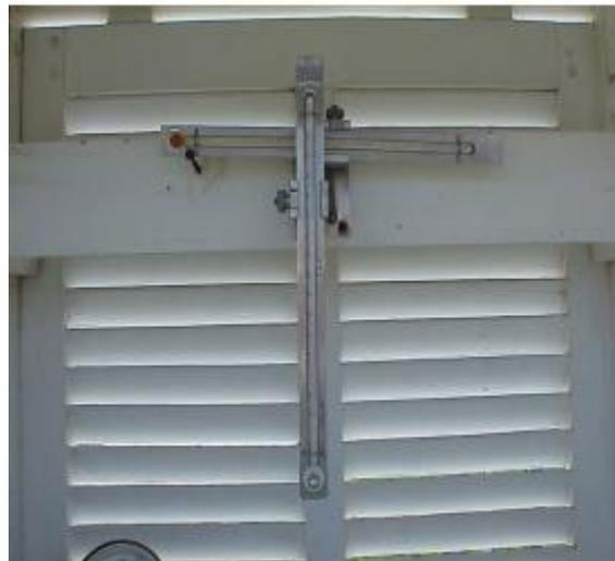
Figure B-30. Maximum Thermometer in Reading Position
