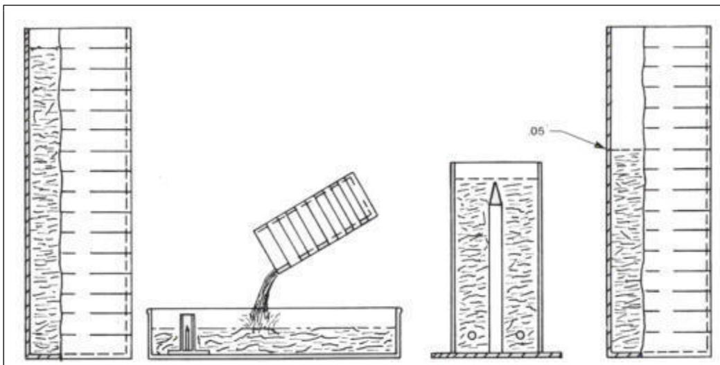
Figure B-36. Fixed Point Gage – Evaporation Measurements
