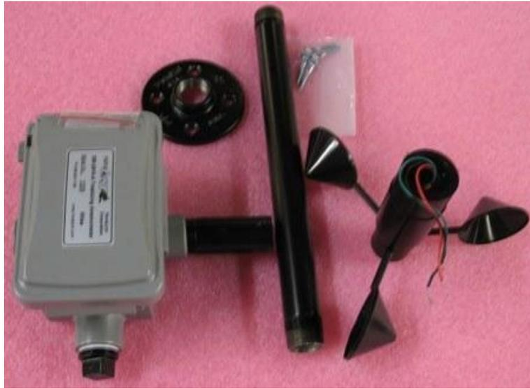
Figure A-27. Totalizing Anemometer (ASN Part F106-1)
