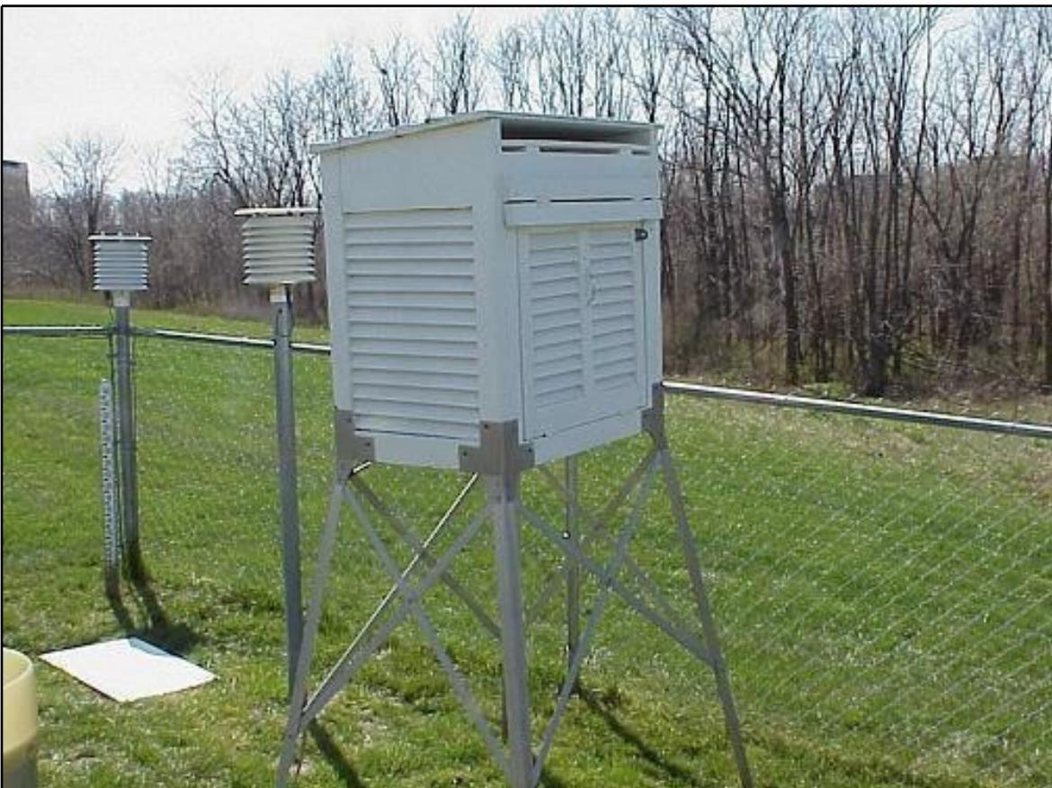
Figure A-12. Instrument Shelters: Cotton Region Shelter and Two MMTS Shelters
