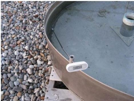
Figure B-40. TW24 Long Stem Max/Min Thermometer
