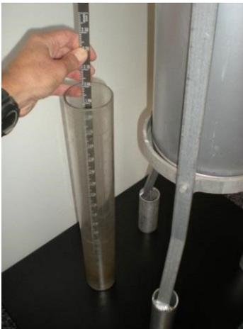
Figure B-11. Dipping the Measuring Stick
