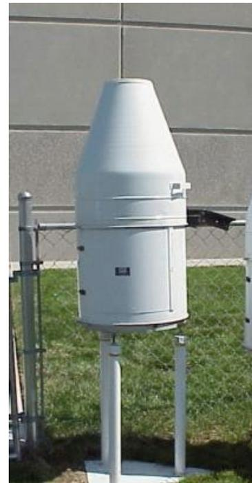
Figure A-10. Fischer- Porter Recording Rain Gauge
