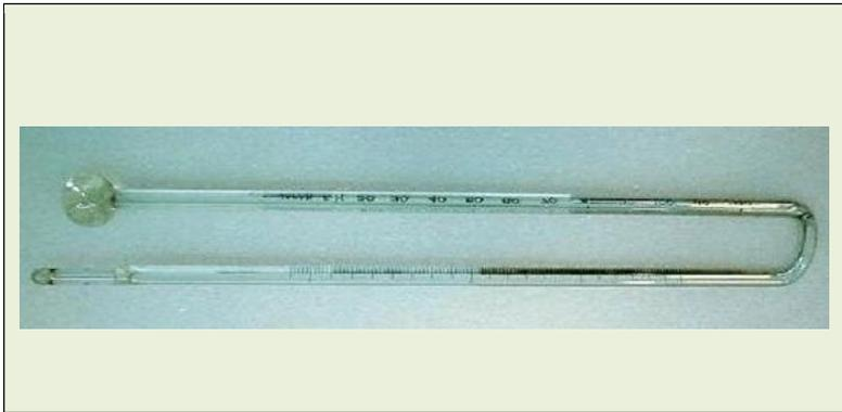
Figure A-28. Six's Thermometer
