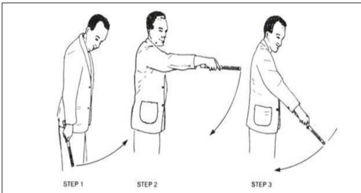
Figure B-33. Joining the Alcohol Column – Centrifugal Method
