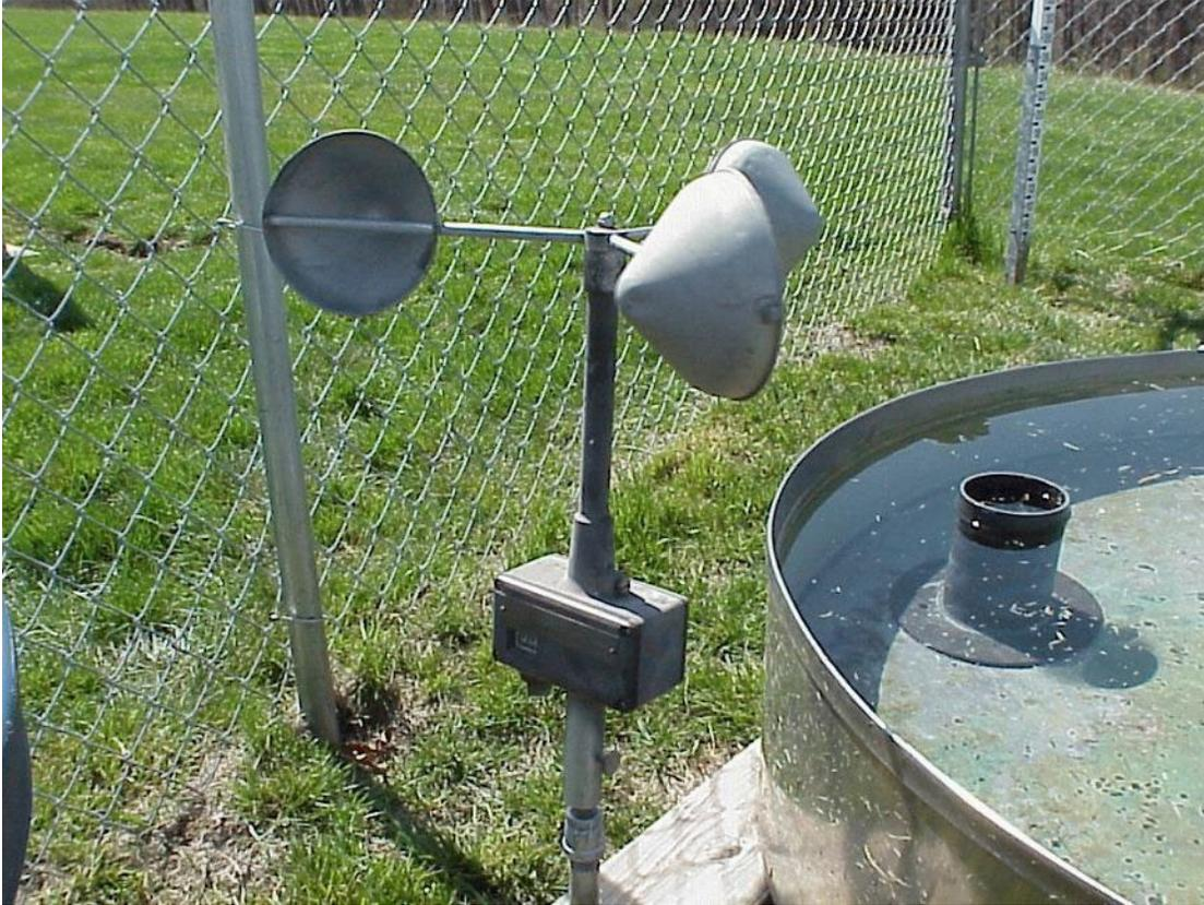
Figure A-25. Totalizing Anemometer (Legacy)
