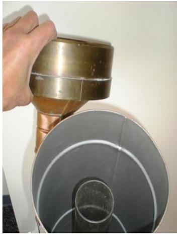
Figure B-9. Removing the Funnel
