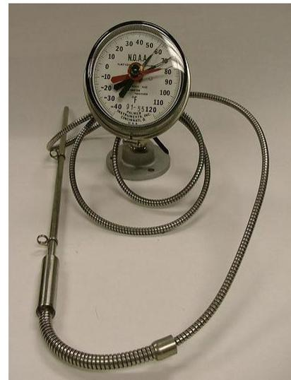
Figure A-35. Palmer Soil Thermometer
