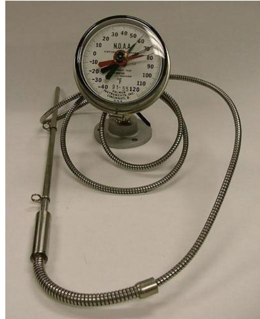
Figure B-44. Palmer Soil Thermometer
