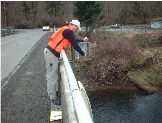
Figure B-46 – Observer at Wire Weight Gauge
