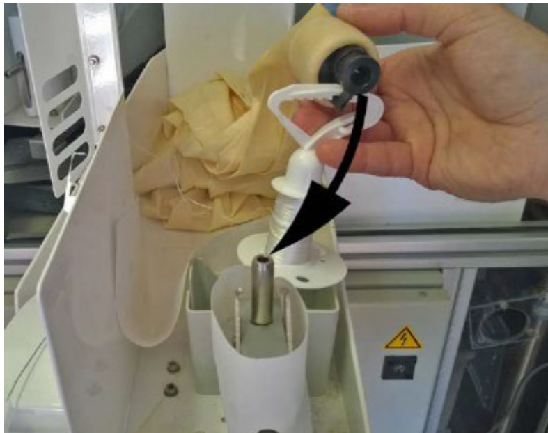
Figure C-23: Snapping the Nozzle on the Nozzle Pipe
