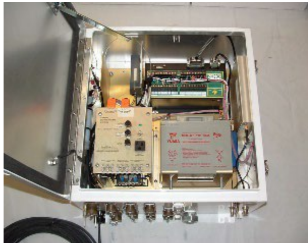
Figure J-7: Remote Processing Unit (RPU)
