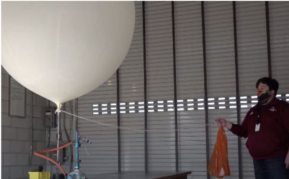
Figure C-5: Completed Balloon Train
