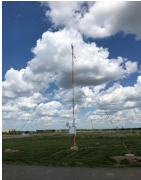
Figure B-6: Vaisala Automatic Weather Station (AWS)
