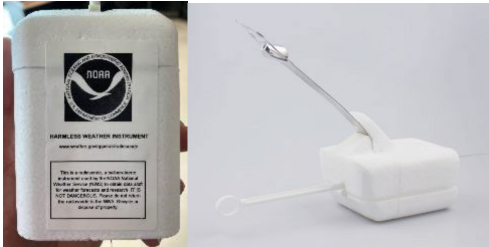
Figure A-1: Upper Air Radiosonde (GRAW)
