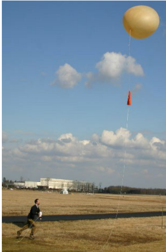
Figure C-7: One Person Release Technique
