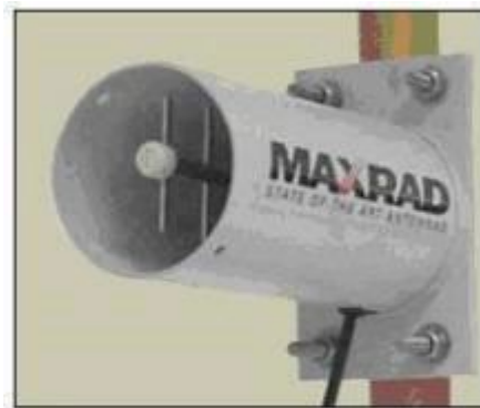
Figure J-9: Yagi Antenna
