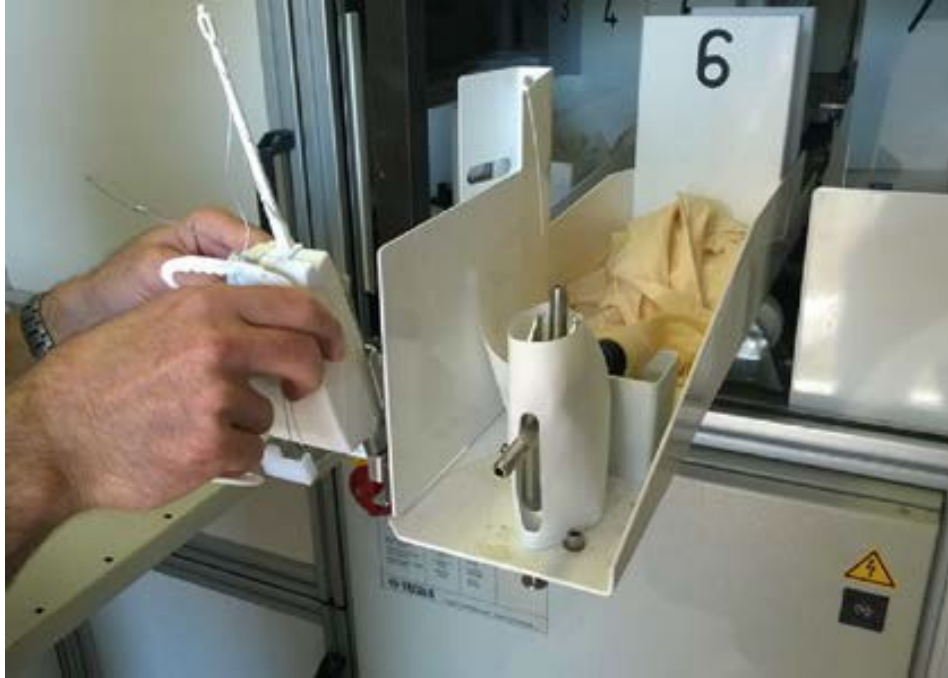
Figure C-18: Placing the Radiosonde in the Holder
