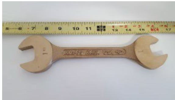
Figure K-15: Typical Brass Non-Sparking Wrench
