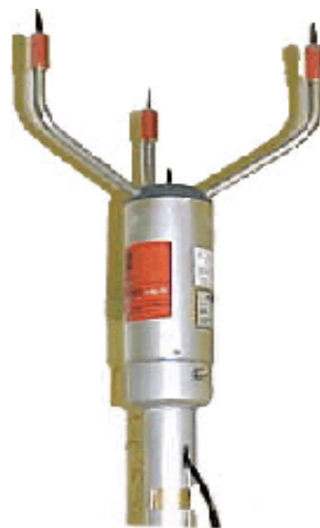
Figure J-3: Vaisala Handar Wind Sensor
