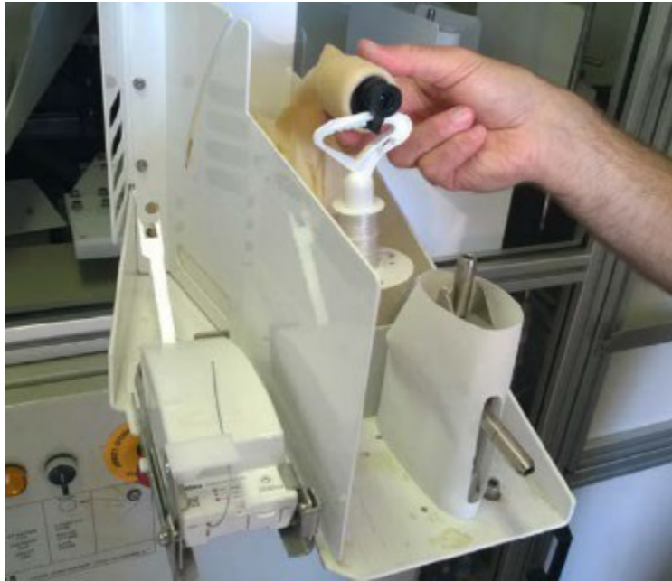
Figure C-22: Unwinder Hook Attached to the Balloon Nozzle
