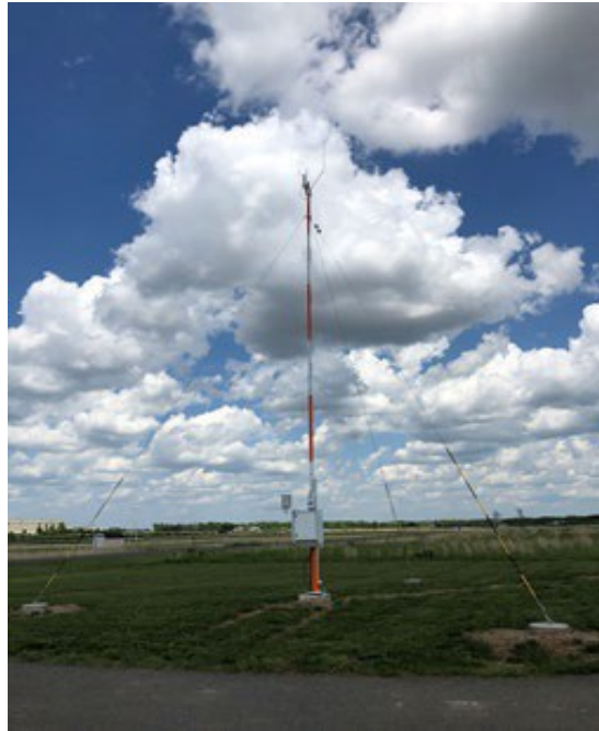
Figure J-10: Automatic Weather Station (AWS)
