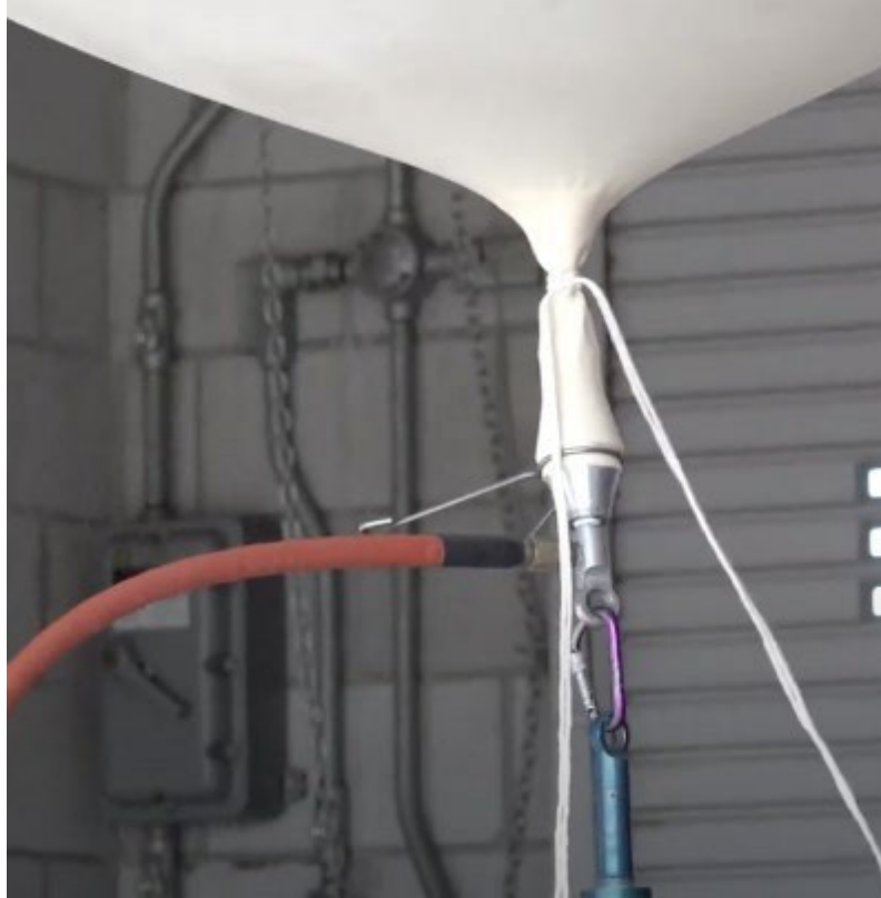
Figure C-4: Balloon Neck Tie-off Post Inflation
