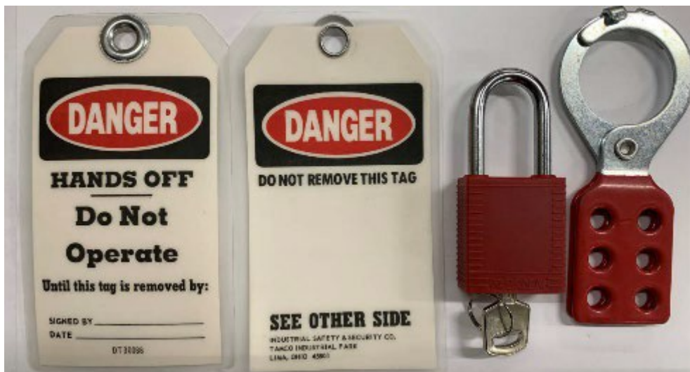
Figure K-19: Lock Out / Tag Out Materials
