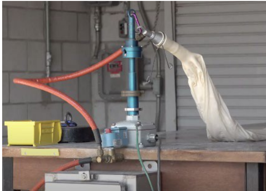
Figure C-1: Balloon on Inflation Table Secured w/Clamp
