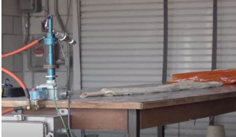
Figure A-5: GP26 Balloon rolled out on inflation table
