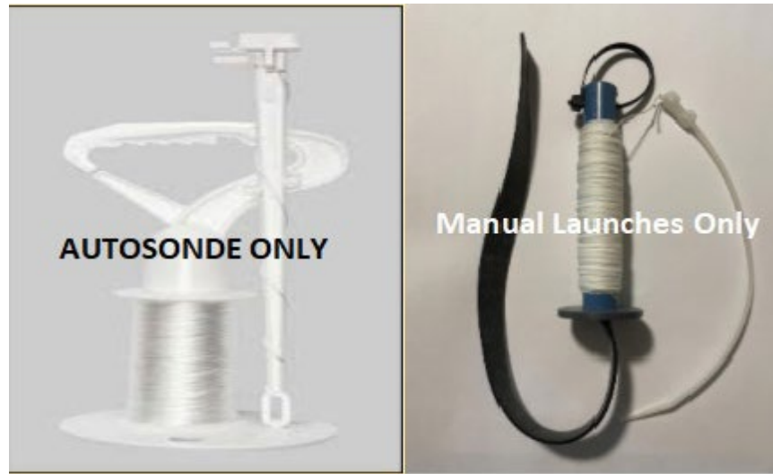
Figure A-6: Types of Unwinders / Dereelers
