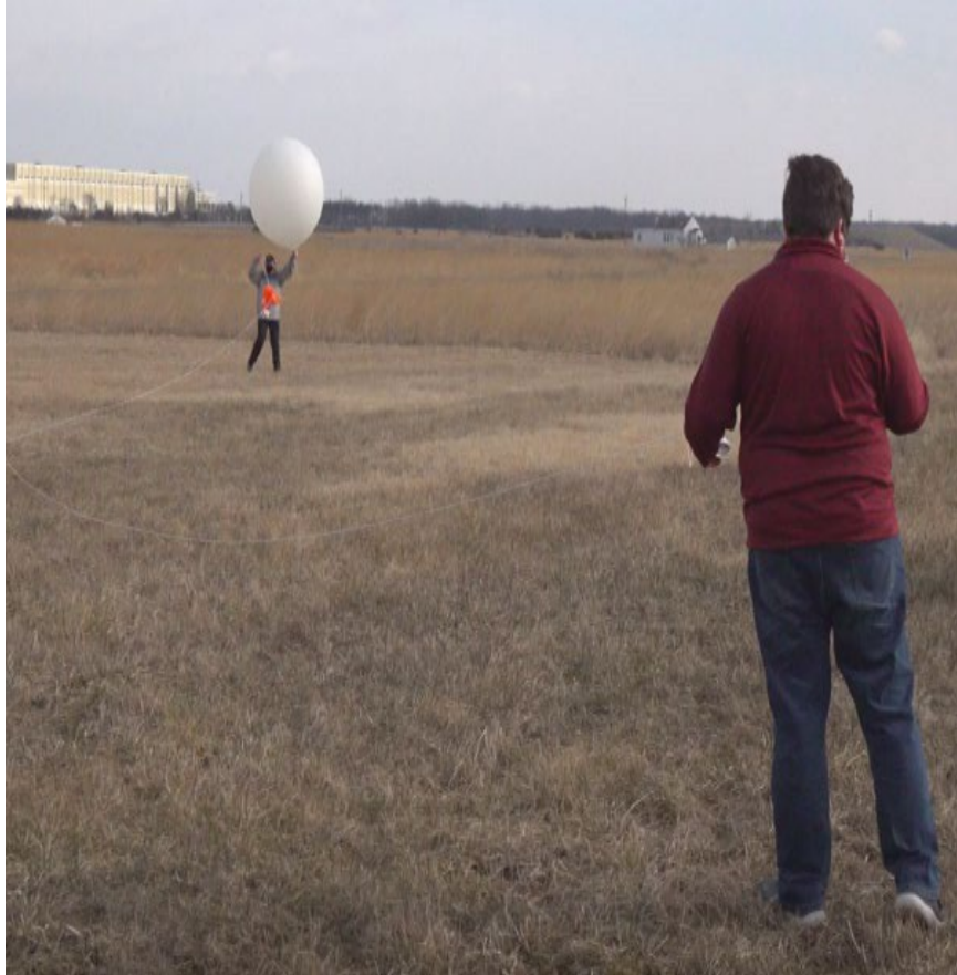
Figure C-8: Two Person Release Technique
