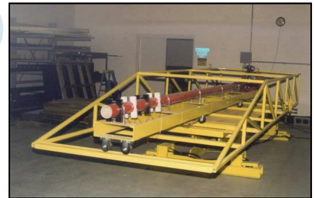
The Wind Science and Engineering Research Center (WISE) at Texas Tech University tests various safe rooms and their components. One test uses this air cannon, which shoots 15-pound two-by-four wooden boards at safe room walls and doors to simulate flying debris. (Photo courtesy WISE)
