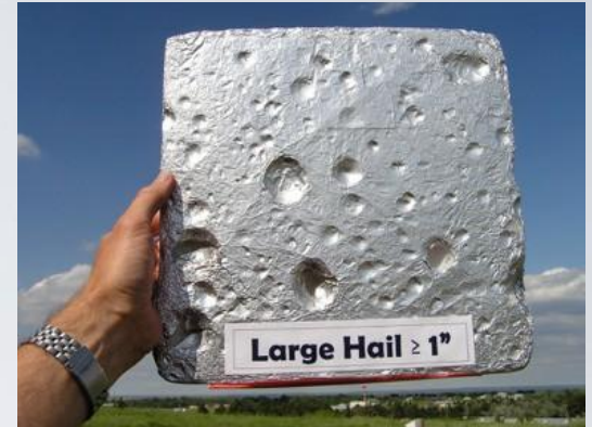
Aluminum foil-wrapped Styrofoam hail pads
