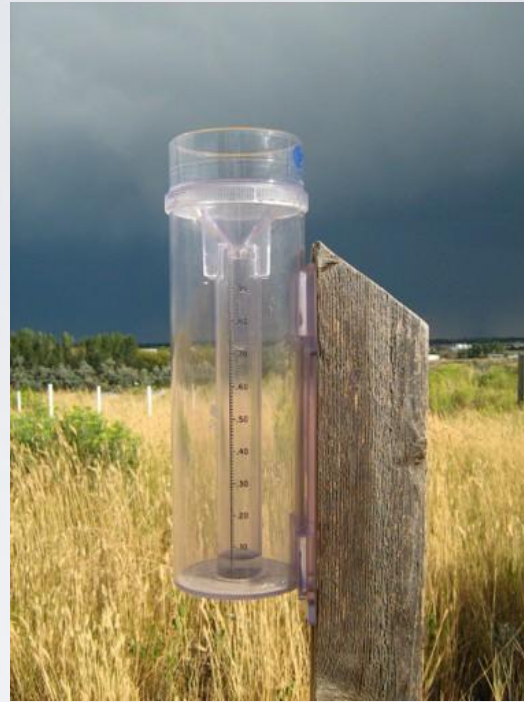
4-inch diameter high capacity rain gauges
