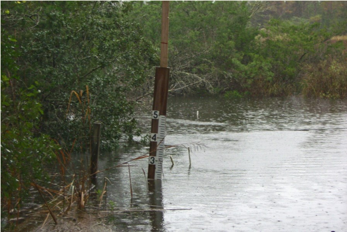
Water level staff gage on Back Creek at the Simpson residence. The red line above the gage is the highest water level during Hurricane Irene in 2011.
