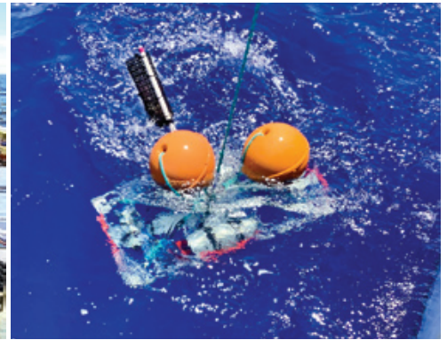
A MOUSS camera system ready for deployment to gather data for the Bottomfish Fishery Independent Survey in Hawai‘i. Photos: Pacific Islands Fisheries Group.
