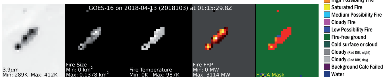
GOES-16 imagery of the Rhea Fire in Oklahoma on April 13, 2018, showing the ABI 3.9 \mu\text{m} shortwave infrared band (left column), and the various outputs of the fire detection and characterization product. From left: fire size, fire temperature, fire radiative power, and fire mask. Fire radiative power is shown in colors from black to red for 0 to 1000 megawatts (MW), red to yellow for 1000 to 2000 MW, and yellow to white for 2000-3000 MW. Credit: CIMSS
