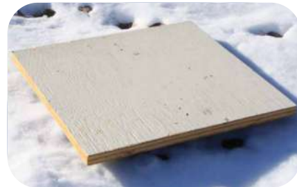
Snow Measuring Board Ex. 16"x16" plywood
