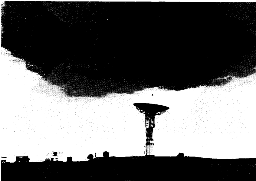
A 10-centimeter radar antenna monitors meteorological developments during the National Hail Research Experiment.
