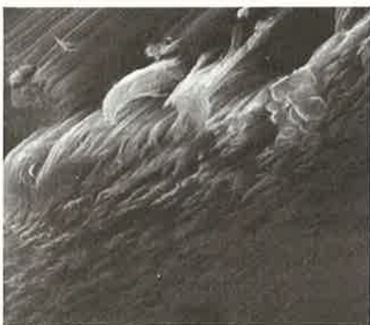
Although the crystal of synthetic polymeric sulfur nitride in the photograph is imperfect (see insert for "perfect" crystal), it illustrates the fibrous nature of the polymer, which, though free of metal elements, behaves optically and electrically as if it were a metal. Subsequent photographs show enlargements of the encircled corner. From top to bottom, the diagram shows how molecules of a sulfur-nitrogen compound ( S_2N_2 ) "open up" by the spontaneous breaking of one of their bonds. They then join with adjacent molecules to form one polymer chain in a crystal of polymeric sulfur nitride (SN)_x . [Photos by University of Pennsylvania]
