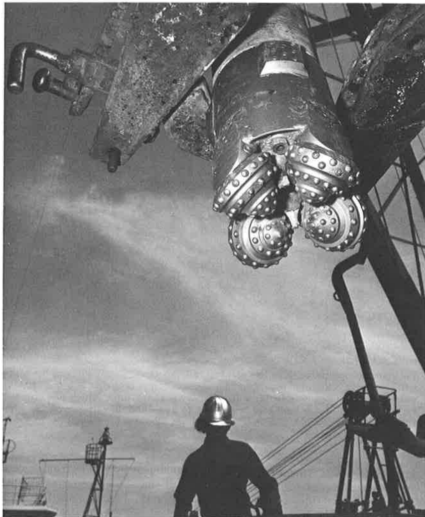
On Leg No. 42 of Deep Sea Drilling Project, an international team of scientists determined that the Mediterranean Sea is at least 65 million years old. This photo shows a core bit, part of the drilling equipment, aboard the ship Glomar Challenger .
