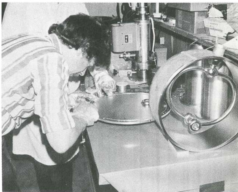
Accelerator booster. Scientists at the California Institute of Technology assemble a "split-loop resonator" intended for use as part of an upgraded accelerator at the State University of New York at Stony Brook. The unusual electricity-conserving device, equipped with 37 of these superconducting resonators, will accelerate heavy atomic nuclei to 10 percent the speed of light, permitting new types of experiments of important physical phenomena.
