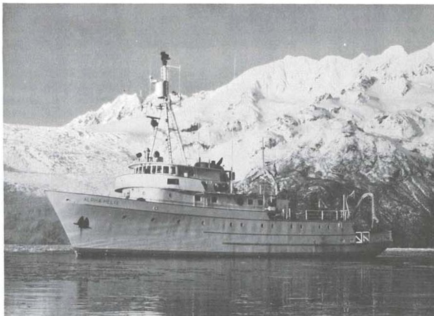
R/V Alpha Helix. This 41.5-meter vessel, part of the U.S. academic research fleet, was once a floating marine biology laboratory. Now converted, the general-purpose research ship can be used in icy seas (photo by Mike Miller). Above, a researcher lowers sampling instruments from the Alpha Helix into the eastern Bering Sea ice pack (photo by H. J. Niebauer).
