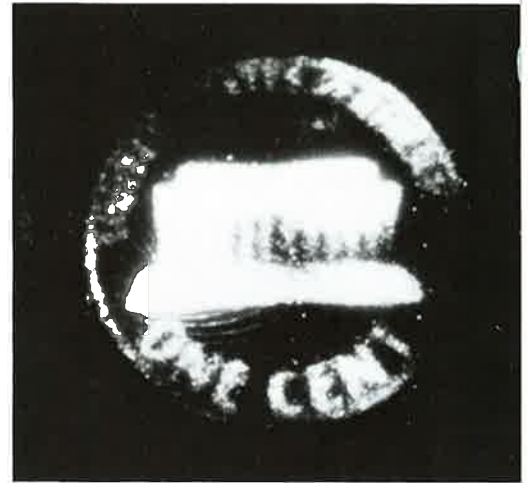
Tactile Sensor Imprint. At the Laboratory for Perceptual Robotics (University of Massachusetts, Amherst), researchers are developing new types of touch sensors for robots. Shown here is a tactile imprint of a penny, acquired by a sensor relying upon optical principles of operation. Tactile and vision sensors are expected to play a leading role in the next generation of robots that can actively sense their environments. Such robots will use that information to control their activities intelligently.
