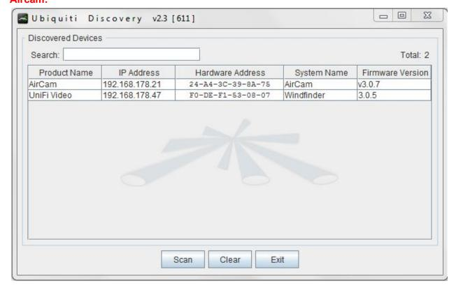
Enter the IP address of the Aircam in the Meteobridge configuration in the field "IP:" (see previous screenshot) and click the webcam symbol again to check if the current webcam view is shown.
