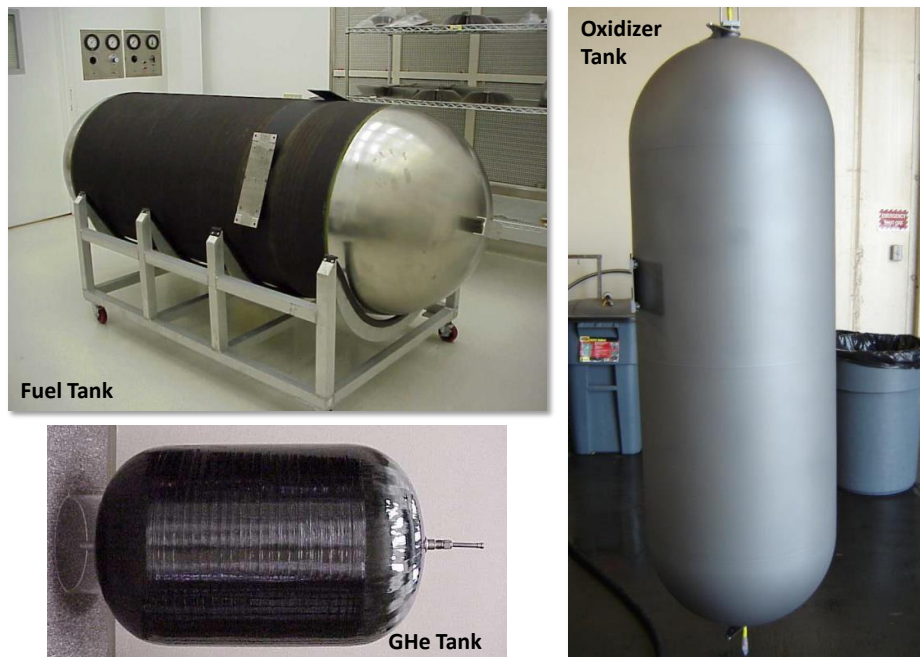
Figure 13-3. GOES-R Series Spacecraft Propellant and Pressurant Tanks
