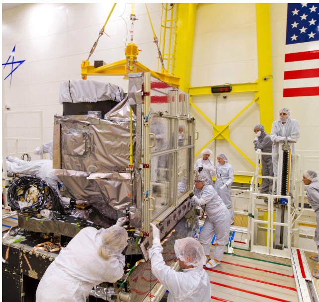
Installation of the GOES-R ABI onto the spacecraft. Credit: Lockheed Martin
