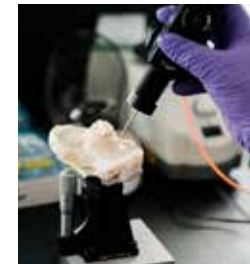
Postdoctoral researcher Masumeh Kazemi (far left) and Michael Albro, an ENG assistant professor of mechanical engineering, use the Raman needle probe on an excised bovine cartilage specimen. Their arthroscope (below) shines light on a specimen, counts the tiny number of light particles that undergo a shift in wavelength, and uses that data to assess the specimen’s chemical composition.
