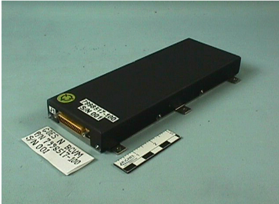
Figure 10-6. Battery Cell Voltage Monitor
