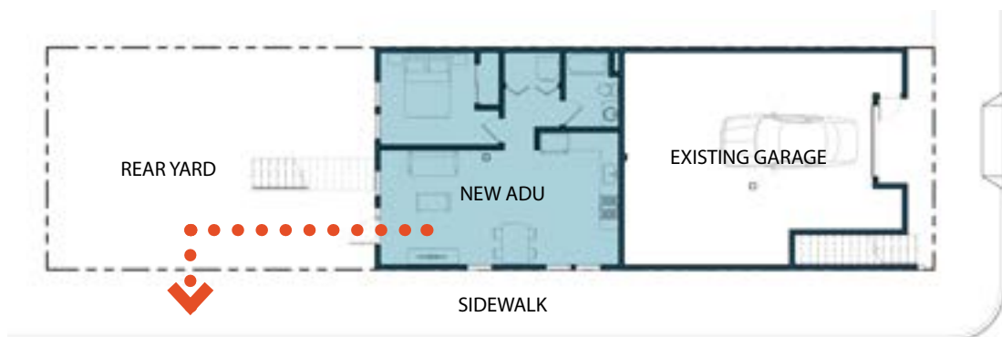
Diagram of Egress Through the Backyard of a Corner Lot
