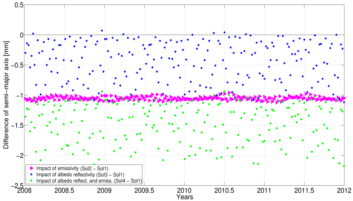
Figure 4.12: Differences of the LAGEOS-2 semi-major axis due to the Earth radiation pressure. The same effect was obtained for LAGEOS-1 (not shown here).
