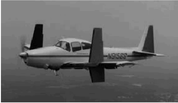
Figure 4: Modified North American Navion A, used to study flight stability (Courtesy Rob Stengel).
