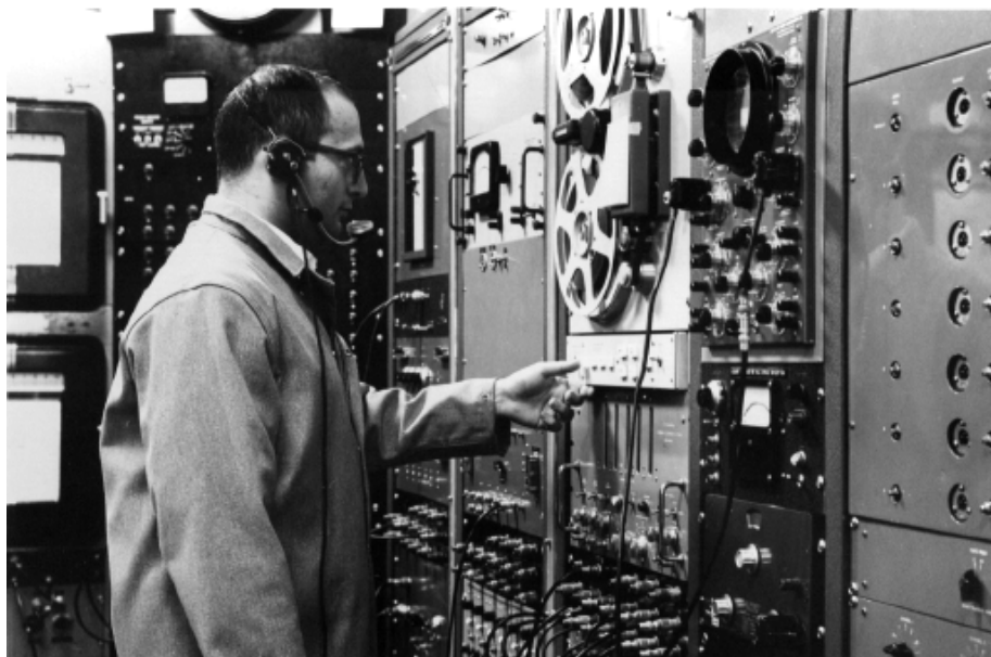
Figure 10: Graduate student W. A. Sirignano*64 prepares equipment to study rapid transients in liquid rocket instability. June 1962.
