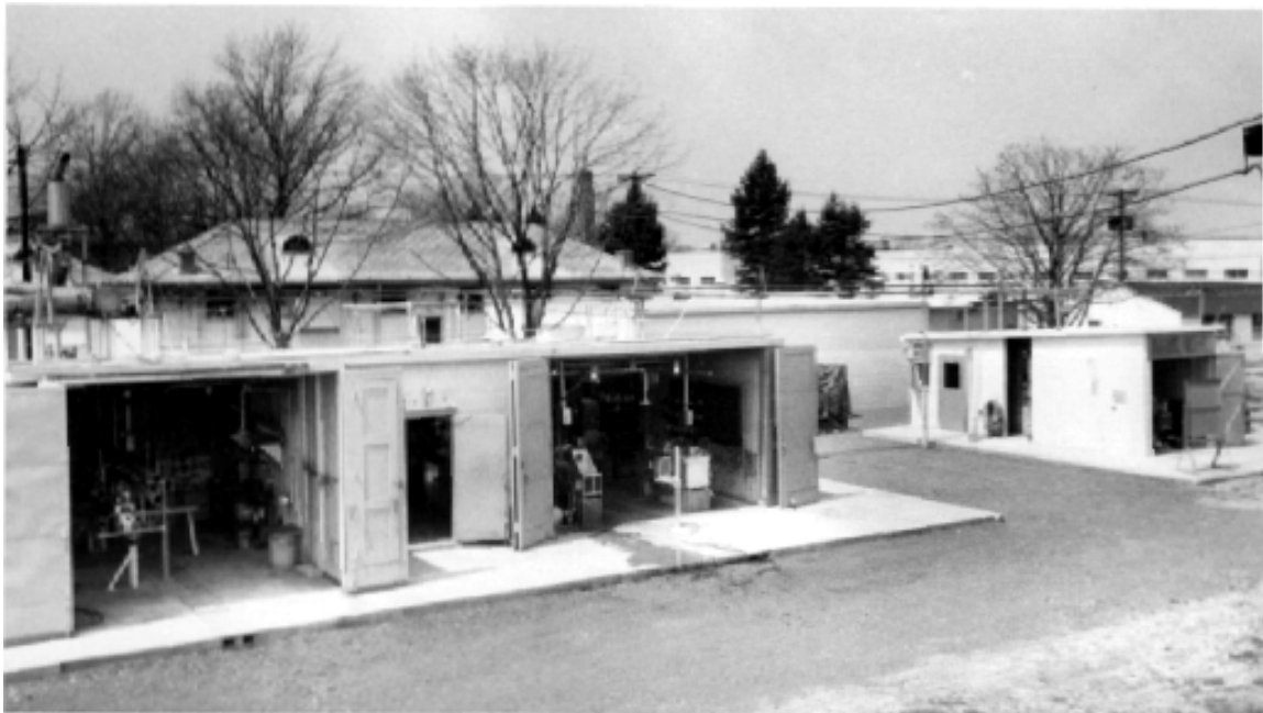
Figure 16: Test cells at Forrester Campus used for studying liquid propellant rocket combustion dynamics. June 1962.
