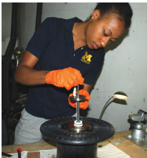
Kimberly Trent assembles a PEPL lab-designed hollow cathode. The hollow cathode is the electron-producing component in Hall Thrusters.
