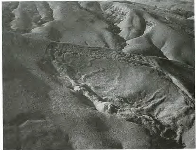
FIGURE 3-26 (above) Shallow translational slide that developed on shaly rock slope in Puente Hills of southern California; slide has low D_r/L_r ratio; note wrinkles on surface [Varnes 1978, Figure 2.33; (Shelton 1966)]. COPYRIGHT JOHN S. SHELTON
