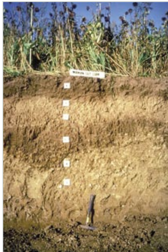
FIGURE 9. Example of soil profile with adequate drainage.
