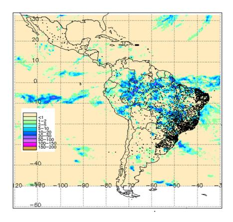
Figure 1: CoSch output for March 3rd, 2000. Black dots represent the position of the raingauges utilized in the combined methodology
