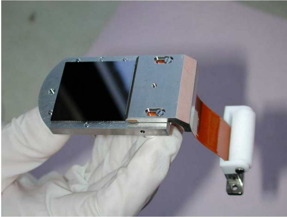
Figure 9-1. SECCHI CCD in its package, with flexprint harness attached. The size of the CCD is about 28.1 mm x 30.3 mm.
