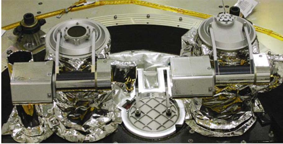
Figure 7-1. Top front view onto the SCIP-B assembly after integration into observatory B. From left to right: COR 1, EUVI and COR 2 doors. The SCIP-A doors are identical.
