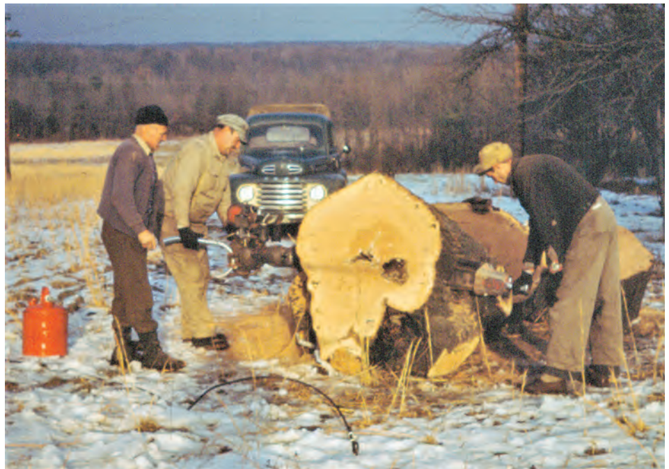
Cutting large log with two-man chain saw, January 1954.
