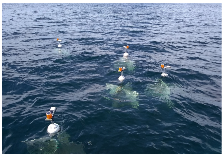
Ocean drifters floating after being released from R/V Endeavor. Drifters include a GPS device, solar powered light, and contact information. Image credit: Wells National Estuarine Research Reserve.
