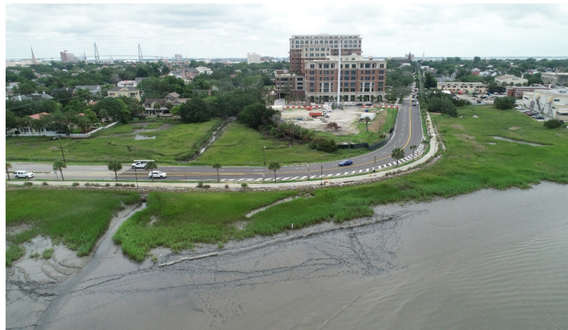
Wire-based living shoreline installed on Lockwood Blvd. Note that a small section of marsh is the only barrier separating the road from the Charleston Harbor. During Hurricane Irma in September 2017, this portion of Lockwood Blvd. experienced severe flooding caused by storm surge from Charleston Harbor. Image credit: SCDNR.
