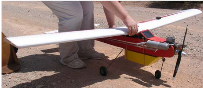
Figure 1. Modified model airplane with yellow cargo pod holding camera, controller and data recorder.
