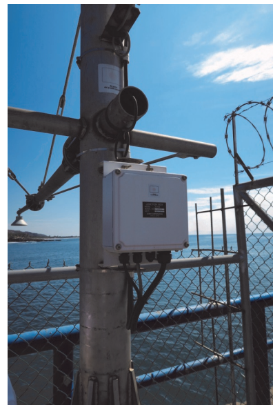
Japanese tide measurement system introduced at a port (El Salvador) Photo: JICA
