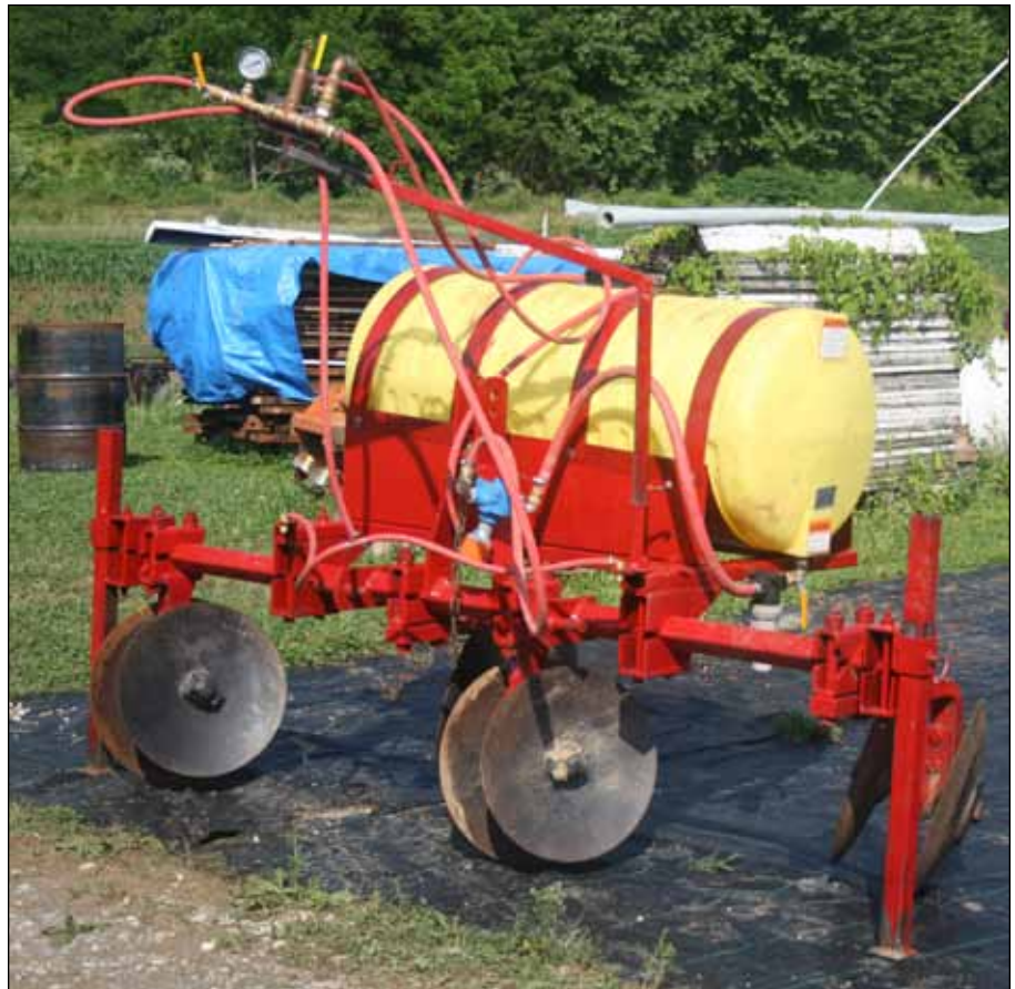
A two-row disk set up to form raised beds for sweetpotatoes. A spray tank and pump has been added to apply insecticide during bed formation.
