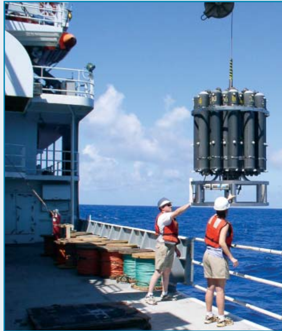
NOAA's Ocean Exploration scientists launch the CTD (conductivity, temperature, depth) over the side of the research vessel Thompson to take ocean measurements.
