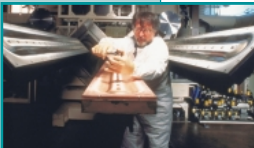
An assembly line employee of CP Films of Martinsville, Va., adjusts a target to a cathode for use in a sputtering machine. The company—which makes polyester films for the defense, automotive, and aerospace industries - received advice from an affiliate of NIST's Manufacturing Extension Partnership.
