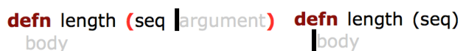
FIGURE 4.2: A use of a placeholder for inserting a new argument [119]. After navigating away the placeholder disappears.
