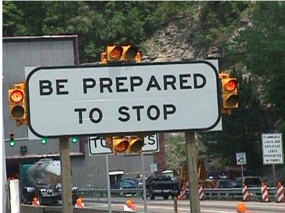
Figure 2.6. Active Warning Sign
