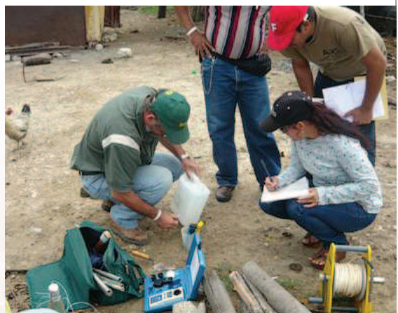
PHOTO 27 Use of a water kit to assess quality in a pond, Cuba
