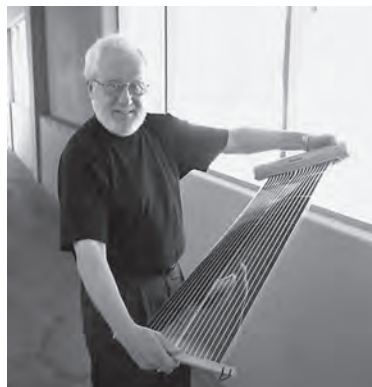
Fig. 1. Solar module, printed on a roll-to-roll tool similar to a printing tool. Its advantages over standard solar cells are flexibility, light weight, low cost, and potential for mass production. (Source: A. Heeger)
