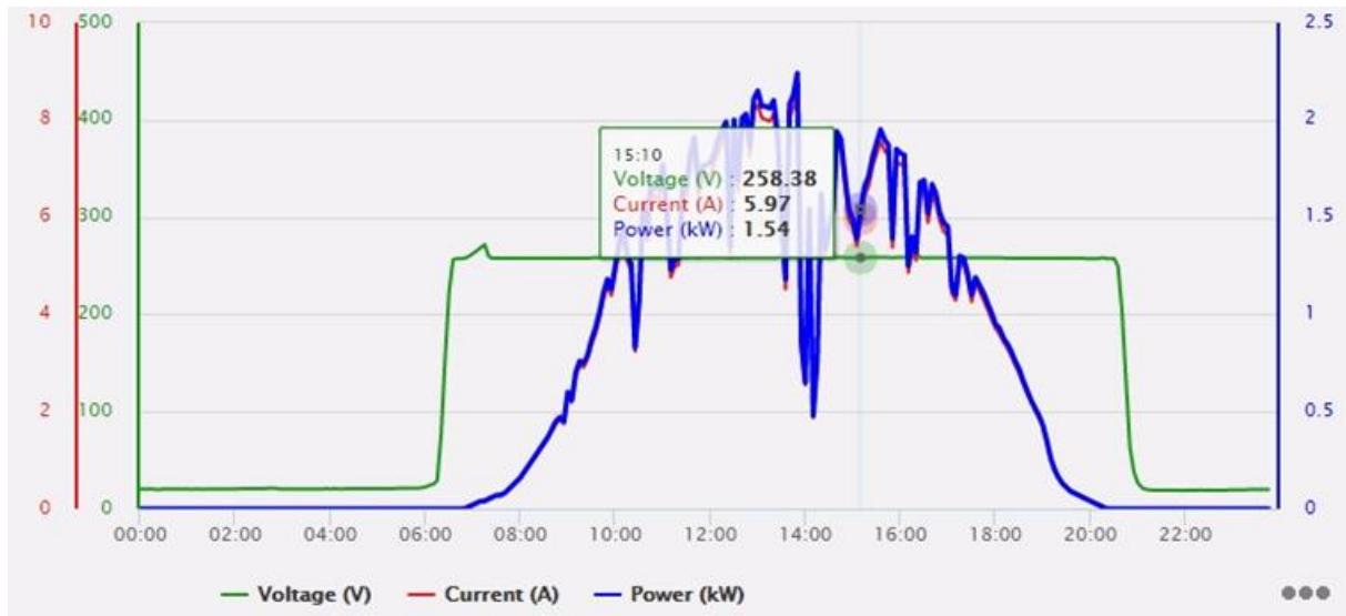
Figure 3. A typical data analysis for the PV production, on a selected date, as shown on web.
