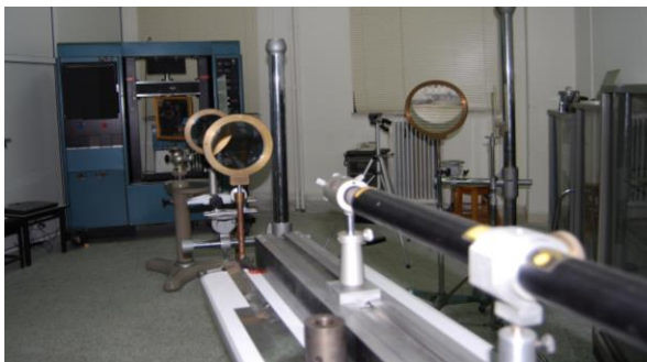
Figure 1. Reflected caustics' experimental set-up.
