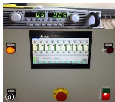
Figure 2. (a) Control System and (b) corrosion cells for the electrochemical corrosion tests.
