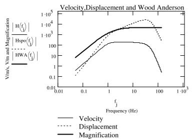
In the plot the amplitude response for Velocity, Displacement and Wood Anderson is shown.
