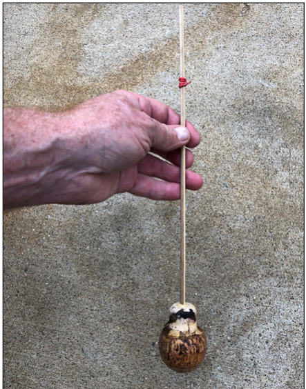
Figure 9. Homemade water level gauge.
